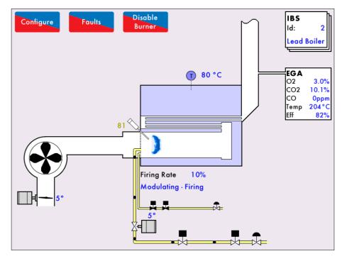
When burning natural gas, the  $CO_2$  value is calculated to be approximately 10% when the  $O_2$  is 3%.
