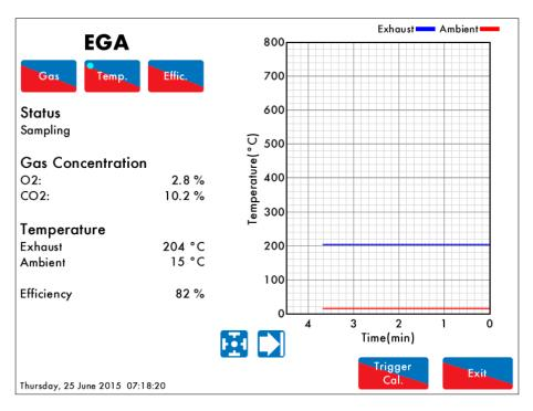
The exhaust gas temperature is related to input 2 on the interface, using a 4-20mA or 0-10V signal. The ambient temperature is taken from input 3 or the default value that is entered when setting up the interface on the PC.
