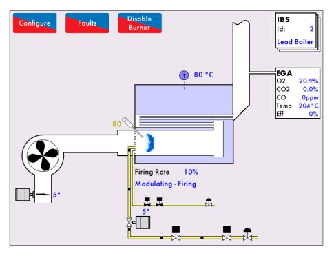
$O_2$  reading shows 20.9% when the 4-20mA or 0-10v signal is maximum (20mA or 10v). The efficiency reading will remain 0% until the  $O_2$  reading is below 19%.
