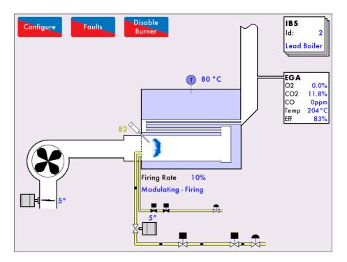
At the minimum reading (4mA or 0v) the maximum CO<sub>2</sub> value will be shown (for  $0\% O_2$ ). This is the value that is set using the PC program as shown in the previous pages.
