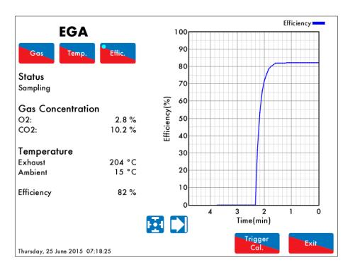
The efficiency can be changed between European and English calculation using the  $O_2$  Interface Configurator software as explained previously.
