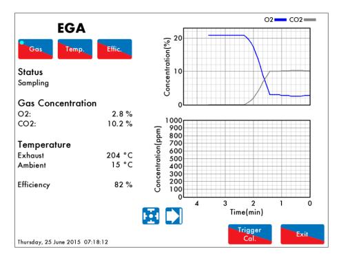
Only the O<sub>2</sub> and CO<sub>2</sub> will be shown and recorded on the Gas history graph. CO is not measured.
