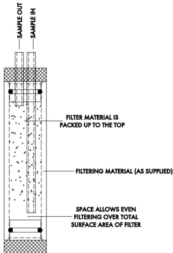
**N.B. FREE SPACE MUST BE LEFT AT BOTTOM TO STOP ANY PREMATURE BLOCKAGE
