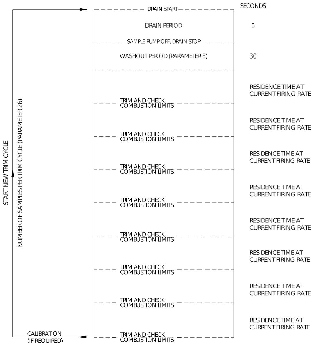
Figure 4.3.4.i Trim Timing Operation
