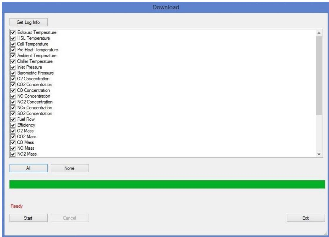
Figure 4.7 ii: selecting and downloading long term data from the EGA
