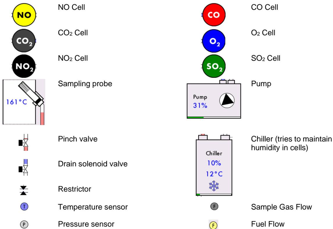
**Note:** The standard cells that are included in the EGA are NO, CO, CO<sub>2</sub>, and O<sub>2</sub>. Optional cells are SO<sub>2</sub> and NO<sub>2</sub>, and they must be fitted at the factory. If the SO<sub>2</sub> and NO<sub>2</sub> cells are not fitted, then the EGA will calculate these values based on the exhaust gases and fuel composition.
