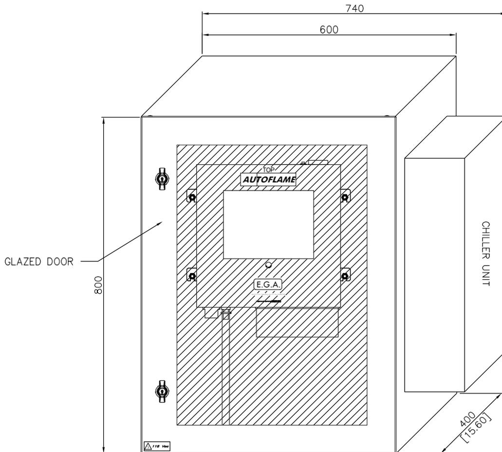
Figure 1.8.3.i Schematic of EGA Chilled Environmental Enclosure
