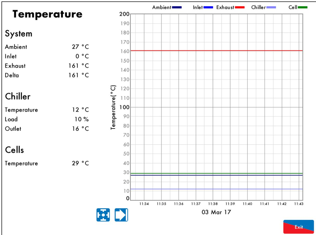
Figure 1.8.4.ii Temperature Screen with Pre-Heated Air Sensor Enabled
